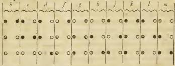
Example. b is denoted by obscuring the upper, and middle lights on the left, and the upper light on the right. c, by obscuring the same lights on the left, and the middle light on the right, and so forth, as expressed against each consonant in the above table.
