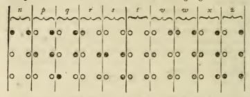
Example. n, is expressed by obscuring the upper and middle lights on the right, and obscuring the upper light on the left, and so forth, as against each consonant expressed in the above table.
