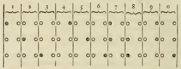
Example. One, is denoted by an obscuration of the upper light, on the left; Two, by an obscuration of the middle light on the left; Three, &c. as expressed in the above table, against each figure, including the cypher.
